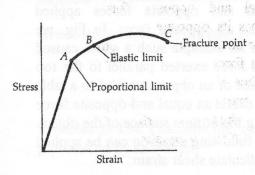
The next figure shows a typical graph of elongation versus applied force. Beyond the proportional limit the graph deviates from a straight line and no simple relationship exists between the force and the elongation. Up to a point farther along the curve called the elastic limit, the object will return to its original length if the applied force is removed. The region from the origin to the elastic limit is called the elastic region. If the object is stretched beyond the elastic
