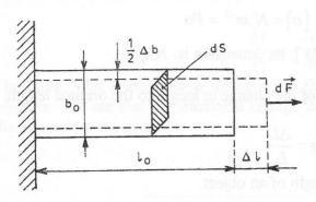
If a force is exerted on an object such as the metal bar in Fig., the length of the object changes. The bar is said to be under **tension or tensile stress**. If the amount of elongation  $\Delta L$ , is small compared to the length of the object, experiments show that  $\Delta L$  is proportional to the force exerted on the object. This proportionality can be written as an equation
