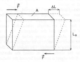
An object under shear stress has equal and opposite forces applied across its opposite faces. In Fig. we have an example such a stress caused by a force exerted parallel to the top surface of an object attached to a table that exerts an equal and opposite force along the bottom surface of the object. The following equation can be applied to calculate shear strain:
