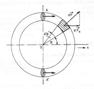
The force component which stresses the flywheel at the chosen cut section A-A' (see Fig.) is equal to
