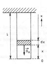
Solution: It is important to bear in mind that the stress along the suspended rope is not constant. At distance x from the free end the stress equals
