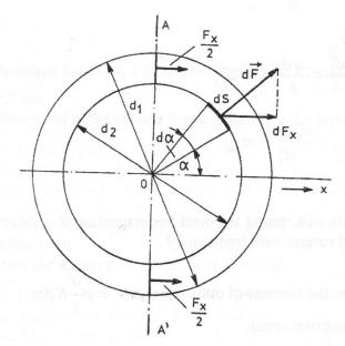
Solution: The force dF = p dS is exerted perpendicularly on the surface element  $dS = \frac{d_2}{2} L d\alpha$ ; when p is the pressure inside the tube and L is its length.
