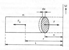
**Problem 1-137.** A uniform rod of length L and density  $\rho$  rotates with constant angular velocity  $\omega$  about an axis passing through its end perpendicular to the rod's axis. Calculate the stress and the extension of the rod.
