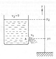
of the liquid as point (2). Assuming the diameter of the vessel is very large compared to that of the hole, the velocity of the liquid surface  $v_2$  will be almost zero. The pressure at both points is the same and it is equal to atmospheric pressure, so  $p_1 = p_2$ .
