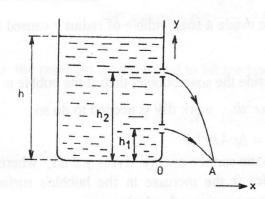
Calculate the height h of the liquid level so that the liquid from both openings falls into the same place A of the plane of the vessel.
