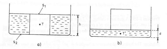
Solution: We shall use the inverse procedure and we immerse the cylinder in a liquid. The original center of mass T' of the liquid will change at position T and the original height of the liquid level d will change to height h (see Figs.)
