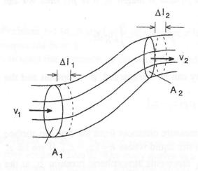
In Fig.,  $v_1$  represents the liquid's velocity as it passes through the cross-sectional area  $A_1$  and  $V_2$  is the velocity as it passes through the cross-sectional area  $A_2$ . The mass flow rate is defined as the mass of liquid that passes a given area per unit time:
