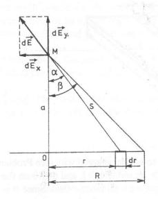
This electric charge sets up an electric field at point M. Due to the symmetry, the components of the electric field parallel to the plane of the disc are cancelled out by an equal but opposite component established by the charge element on the opposite side of the ring. Thus the component of the electric field perpendicular to the plane of the circle contributes to the resultant electric field,
