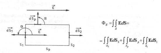
For the left cap, the angle  $\alpha$  for all points is  $\pi$ , the electric field has a constant value, and thus for the flux through the left cylinder cap we can write
