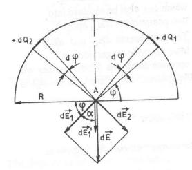
Since symmetrically to the charge  $dQ_1$  is on the ring placed the same charge  $dQ_2$  which produces at point A the electric field  $dE_2$  than the electric field due to these two charges is
