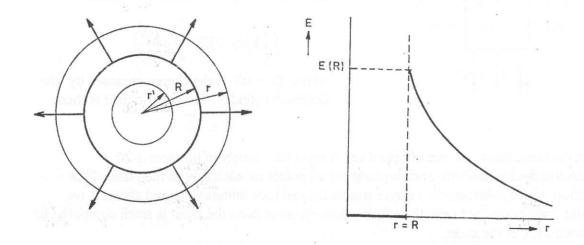
To determine the electric field outside the sphere, we choose as Gaussian surface a sphere of radius r(r>R). As long as the electric field on this sphere is constant we obtain from Gauss' law:
