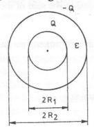
$$U = \int_{R_1}^{R_2} E \, dr = \frac{Q}{4 \, \pi \, \varepsilon} \int_{R_1}^{R_2} \frac{dr}{r^2} = \frac{Q}{4 \, \pi \, \varepsilon} \frac{R_2 - R_1}{R_1 \, R_2}$$
