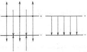
Solution: We can solve this problem using the superposition principle. In the region between the plates, the fields of the two plates are in the same directions. Adding the parallel vectors, we obtain
