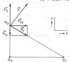
We resolve force  $\mathbf{F}_1$  into its components along the x and y axes as shown:
