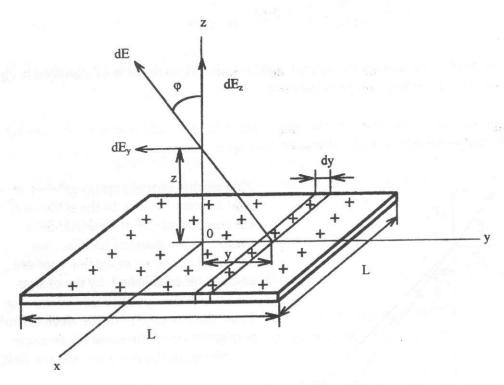
Solution: Since we already know the electric field due to a long charged wire (see Problem 3-17), let us divide the plane into long narrow strips of width dy and length L and then sum the contributions to the electric field due to each strip to get the total electric field. Since  $\sigma$  is the surface charge density the charge on each strip is
