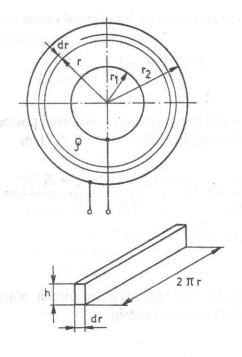
b) To determine the resistance of this resistor in which the current flows radially outward we divide the resistor into concentric cylindrical shells (see the figure) and then we integrate it from radius  $r_1$  to radius  $r_2$ . The length of each elementary conductor is dr and its cross-section is  $(2\pi rh)$ . Thus we have
