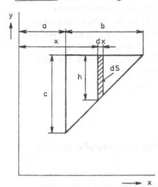
the magnetic flux  $d\Phi$  passing through the elementary area dS. In this area the magnetic induction can be considered to be a constant. Thus the magnetic flux through the area dS is
