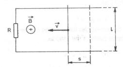
a) Disregarding the magnetic field due to the current in the conductor the induced electromotive force is
