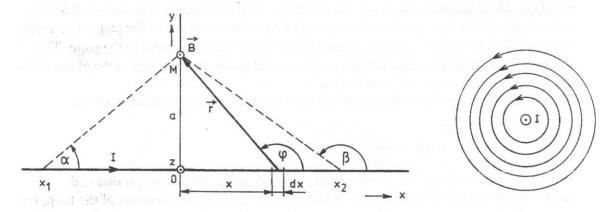
Consider an infinitesimal current element I.dl = I.dx.i located at a distance x from the y axis. The displacement vector r from this current element to the field at point M is
