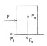
When an object is at rest on a table the gravitational force does not disappear. From the second law of motion the net force on an object at rest is zero. There must be another force on the object to balance the gravitational force. For an object resting on a table, the table exerts this upward force and this force is usually referred to as the **normal force**  $\mathbf{F}_N$ .
