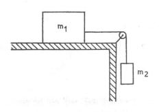
friction is equal to  $\mu$ . Another body of mass  $m_2$  is freely hung over a pulley and is coupled to mass  $m_1$  by means of a rope whose mass is not taken into account. The mass of the pulley is also disregarded.
