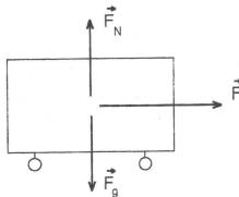
Solution: There are three forces acting on the cart. The forward pushing force  $\mathbf{F}_p$ , the downward force of gravity  $\mathbf{F}_g$  and the upward force  $\mathbf{F}_N$  exerted by the floor. Since the cart is not accelerated vertically the sum of both vertical forces must be zero. Then the net force on the cart is simply  $\mathbf{F}_p$ .
