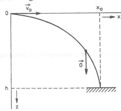
Solution: The origin of a co-ordinate system is set into the starting place of the motion. At any moment of the motion there is the only force acting on a projected object - the force of gravity  $\mathbf{G}(0,0,\mathrm{mg}) = \mathrm{mg}$  when m is the mass of the object.
