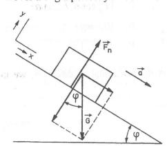
Solution: There are two forces acting on the object in the chosen co-ordinate system: the force of gravity  $\mathbf{G}(\text{mg sin}\alpha, -\text{mg cos}\alpha)$  and the normal force  $\mathbf{F}_N(0, F_N)$ .
