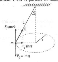
**Problem 1-40.** A particle of mass m suspended by a cord of length L revolves in a circle of radius  $r = L \sin \varphi$ , where  $\varphi$  is the angle the cord makes with the vertical (see Fig.). Calculate the speed and period of its motion.
