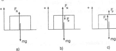
a) The weight of the box is mg. If we have chosen an upward direction as positive the net force on the box is  $F = F_N - mg$ ; where  $F_N$  is the normal force exerted upward on it by the table. Since the box is at rest, the net force on it must be zero, thus
