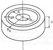
Solution: We divide the cylinder into concentric cylindrical rings of thickness dR. The mass of such a ring equals  $dm = \rho dV$ , where  $\rho$  is density and  $dV = 2\pi R dR h$  is its volume.
