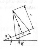
**Problem 1-121.** There is a squared pyramid on an inclined plane, as shown in Fig. Its height is h and the edge of its base has a magnitude of a.
