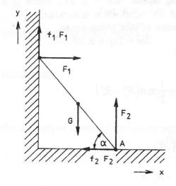
the ladder does not fall due to its weight. (see Fig). The coefficient of friction between the wall and the ladder is  $\mu_1$  and between the ground and the ladder is  $\mu_2$ .
