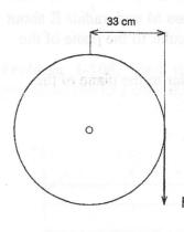
Solution: The net torque is the applied torque due to  $F_T$  minus the frictional torque
