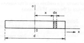
Solution: Since the axis is through the center of mass of the stick, the integration extends from -d/2 to +d/2. Thus
