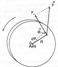
Let us now calculate the work done on a body rotating about a fixed axis. We suppose that a force F acts at a point at a perpendicular distance R from the axis of rotation.
