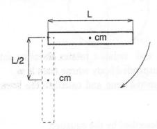
Solution: We can use the work-energy theorem here; the work done is due to gravity. The work done by gravity is, of course, equal to the change in gravitational potential energy of the rod. Since the center of mass of the rod drops a vertical distance L/2, the work done by gravity equals
