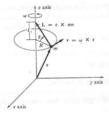
For a rigid body, then, in which all particles  $m_i$ rotate with the same angular velocity ω about an axis of rotation that is fixed with respect to the body, the angular momentum of the body along the axis of rotation is
