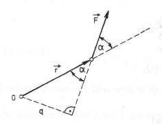
Firstly, we define the moment of a force. If a force  $\mathbf{F}$  acts on a simple particle at a point whose position with respect to the origin 0 of the inertial reference frame is given by the position vector  $\mathbf{r}$ , the torque  $\tau$  acting on the particle with respect to the origin 0 is defined as the vector product
