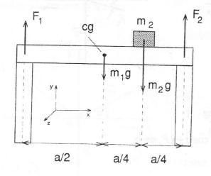
Solution: The weight of the beam acts at its center. The force the beam exerts on the supports is equal and opposite to the forces exerted by the supports on the beam.
