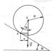
Solution: When the sphere rolls without slipping, the point of contact moves the distance  $s = R.\alpha$ , which is the distance moved by the sphere's center.
